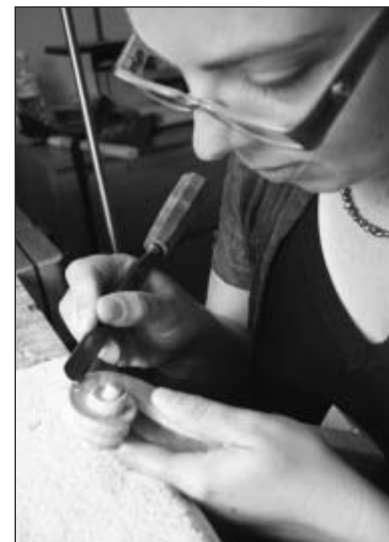
INTRICATE DETAIL: Yankovich uses a small carving tool to form a piece of wood into a violin scroll. (Photos by Marcia Downham)
